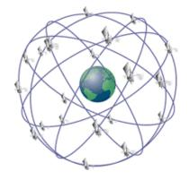
Figure 9 - GPS Satellite Orbits
